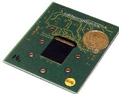
Fig. 1. A MIMOSA 5 sensor glued on a PCB adapter board.
