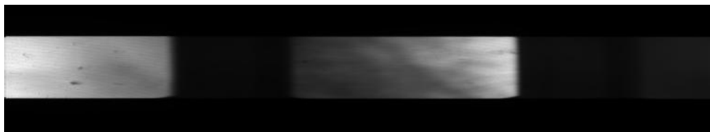
Figure 6. Sample image of H- \alpha showing an image with the wavelength 6563.3 Å in the middle and two adjacent ghost images at 6563.3 \pm 3.74 Å
