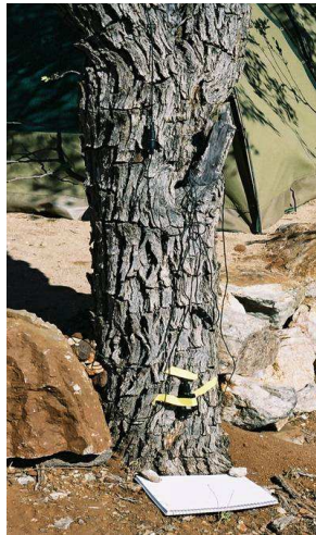
Fig. 1. Middle School students helped design an experiment to measure changes in light intensity and temperature during totality. A light sensor attached to a tree and trained on a white piece of paper measures the reflected light throughout the eclipse. The temperature probe was kept in the shade on the other side of the tree.
