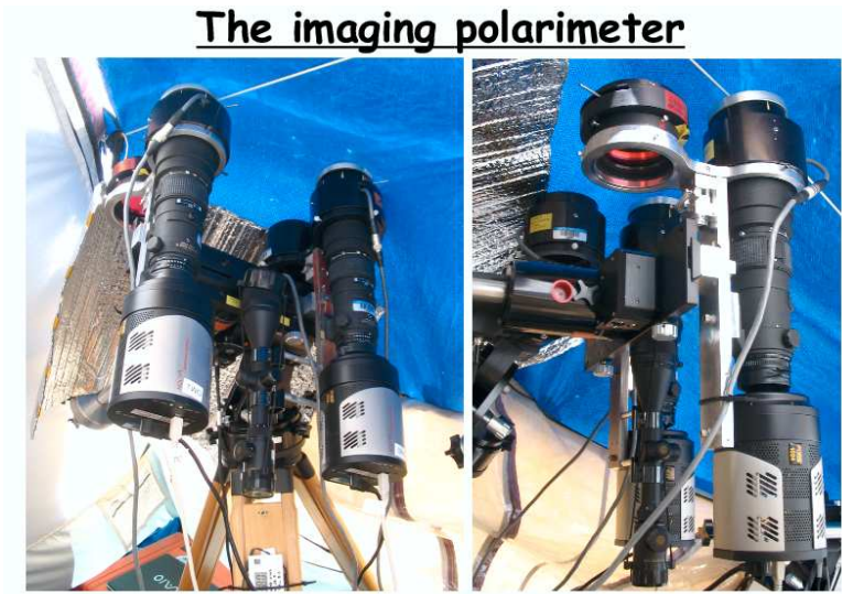
Fig. 4. Two views of the imaging polarimeter from within the observing tent. Two PIXIS 1024BR cameras are mounted on the same German Equatorial mount, with filters attached to each camera. The filters could be interchanged during the observing run. The polarizers were manually controlled.
